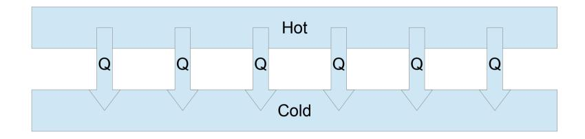
2<sup>nd</sup> Law of Thermodynamics Heat travels from hot to cold (until the temperatures are identical)
